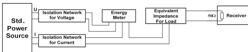
Figure 2. Impedance variation test
