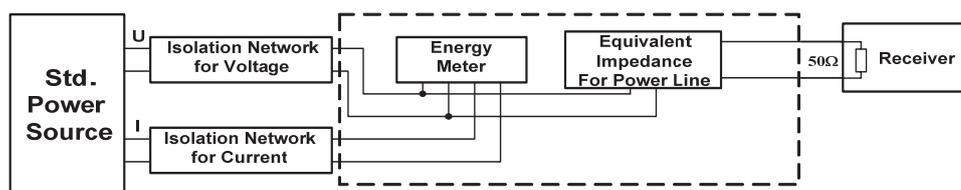
Figure 3. Noise disturbance test
