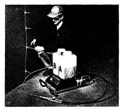
Liquid Control's Posiratio® Mini crack-injection dispenser is ideal for concrete restoration projects. It is specially designed to simply, accurately and inexpensively inject epoxy into concrete cracks.
