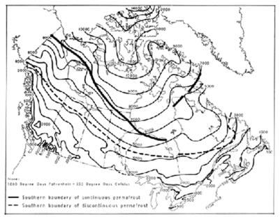
*Figure 1. Normal Freezing Index for Canada in degree days Fahrenheit based on the period 1931 to 1960 (Boyd, 1973).*
