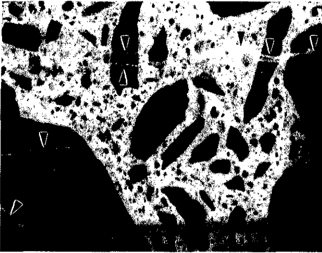
Fig. 3(a)—Optical micrograph of gel filling cracks (indicated by arrows) in limestone aggregate particles and paste; scale divisions in 0.5 mm. (0.02 in.)
