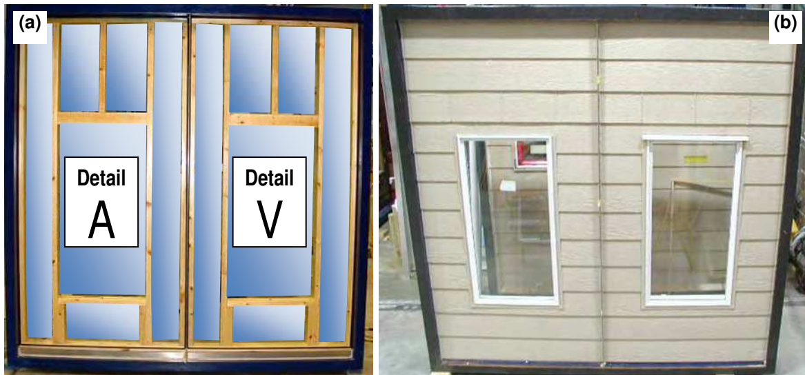
Figure 1 — (a) schematic of front elevation of 2.44-m by 2.44-m (8-ft. by 8-ft.) specimen showing location of 600 mm by 1200 mm (2-ft. by 4-ft.) windows and adjacent wood framing studs. Detail “A” might be representative of installation details used in current practice whereas detail “V” a variation on that practice; (b) photo of a completed specimen clad with hardboard siding
