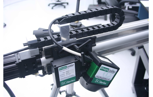
Figure 2. SG-series laser line scanner mounted on a translation stage
