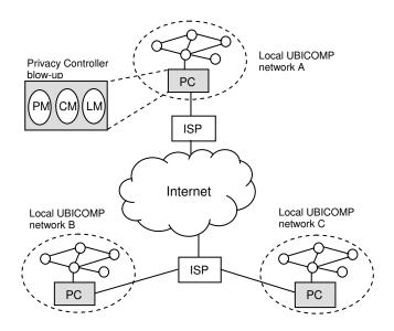
Figure 4. Privacy-Preserving UBICOMP architecture (ISP = Internet Service Provider, small circles are UBICOMP devices, PC = Privacy Controller, PM = Policy Module, CM = Compliance Module, LM = Link Module).
