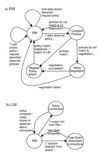
Figure 5. High level state machines illustrating the behavior of the PM and LM components of the Privacy Controller.
