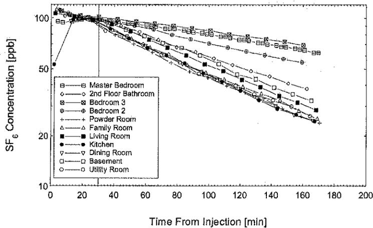
Figure 7b Simultaneous room-by-room decay measurements for configuration A at  $+11^{\circ}\text{C}$ . Local exhaust system—vents sealed.
