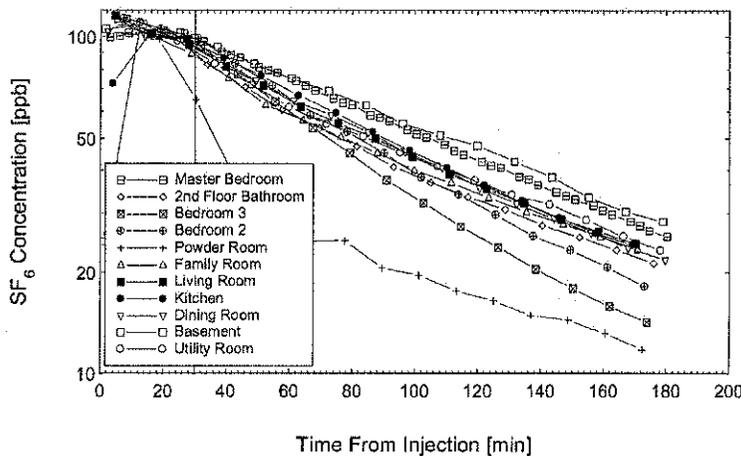
**Figure 11b** Simultaneous room-by-room decay measurements for configuration E at  $+12^{\circ}\text{C}$ . Minimal ducted supply system with local exhaust system—no vents.
