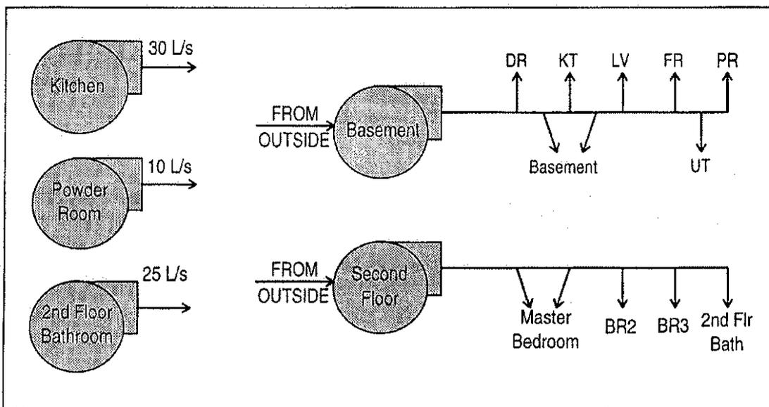
Figure 4 Schematic illustration of minimal ducted supply system—configuration E.
