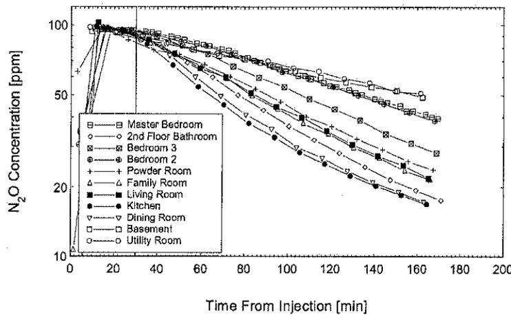
**Figure 10b** Simultaneous room-by-room decay measurements for configuration D at  $+12^{\circ}\text{C}$ . Partially distributed exhaust system—vent open.
