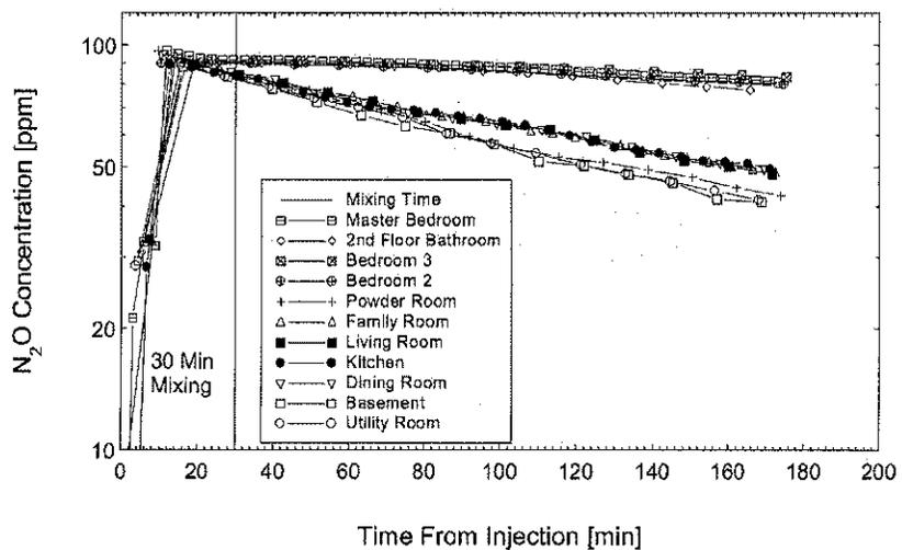
**Figure 5** Simultaneous room-by-room decay measurements for configuration F at -13°C. Reference case - windows and vents sealed, fans off, furnace fan off.
