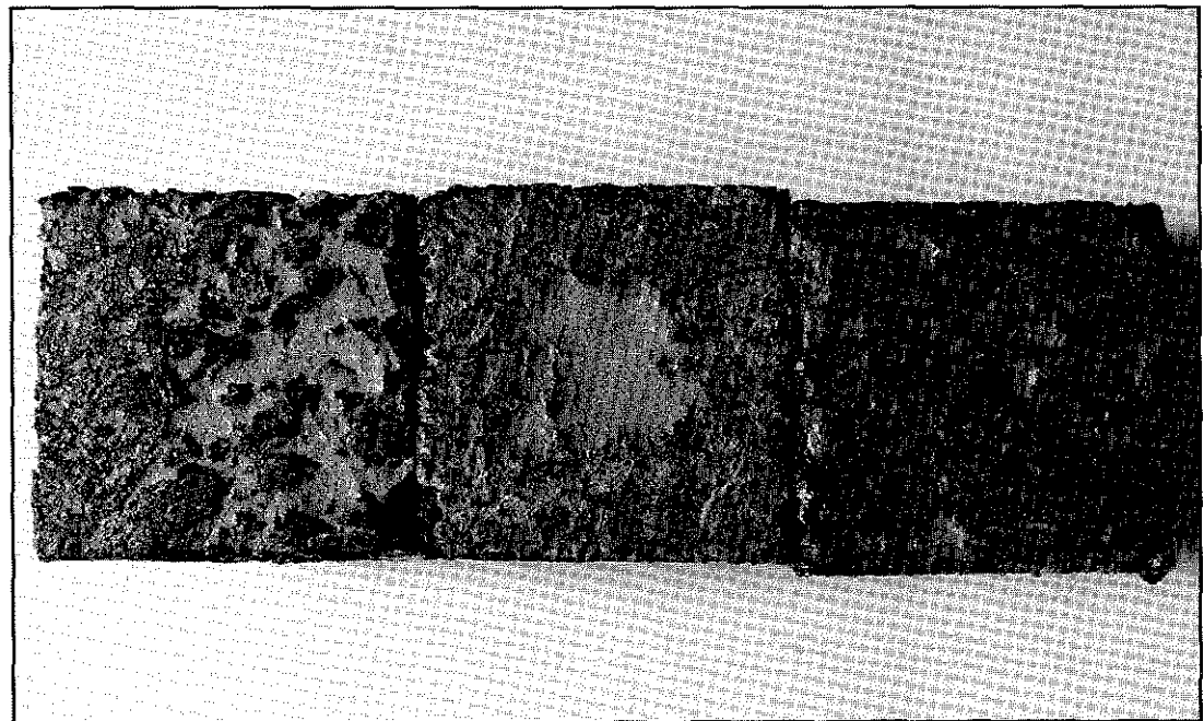
Figure 19. Surface of AC briquettes after tensile tests on sealant-briquette assemblies when the briquette is untreated (middle) and overheated (left). On the right, is the briquette surface without sealant. The briquettes were covered with dyed paste to increase the contrast between the holes in the briquette and the unaltered surface. On the untreated briquette, the sealant pulls out aggregates from the surface, leaving a hole in the middle of the briquette. On the overheated surface, there is no hole where the sealant was adhering. Instead, small holes are scattered across the surface where the hot-air lance caused damage.
