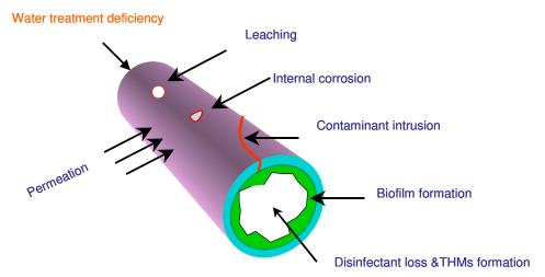
Deterioriation mechanisms in distribution networks causing risk of water quality failures.
