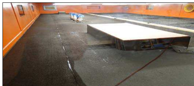
(c) Specimen ready for testing by simulating wind uplift forces
