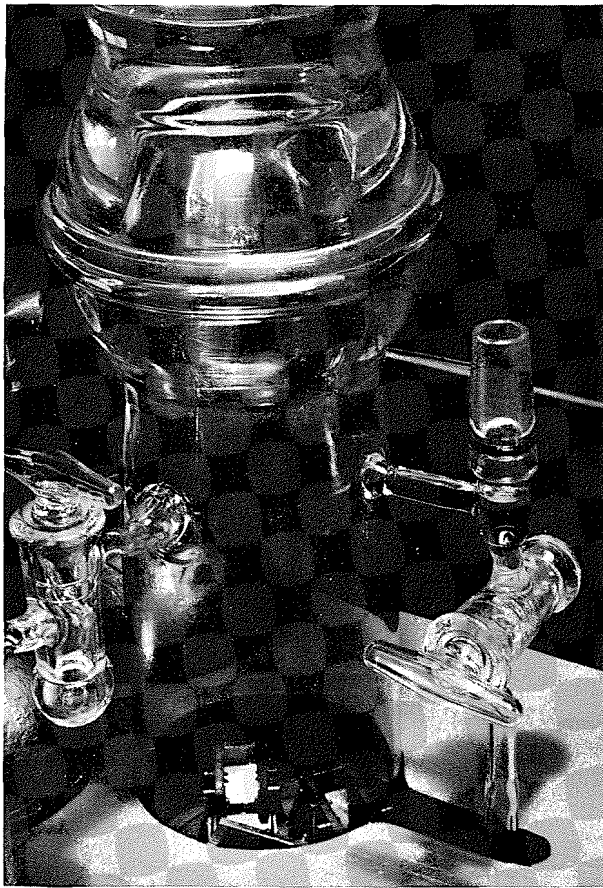
Figure 2: Conditioning cell with optical extensometers and mounted samples.
