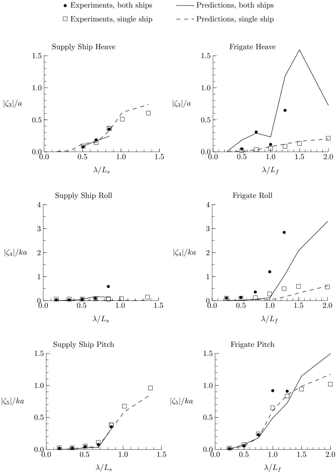
Figure 6: Ship Motions with Frigate 45 m Ahead of Supply Ship, 12 knots, Head Seas
