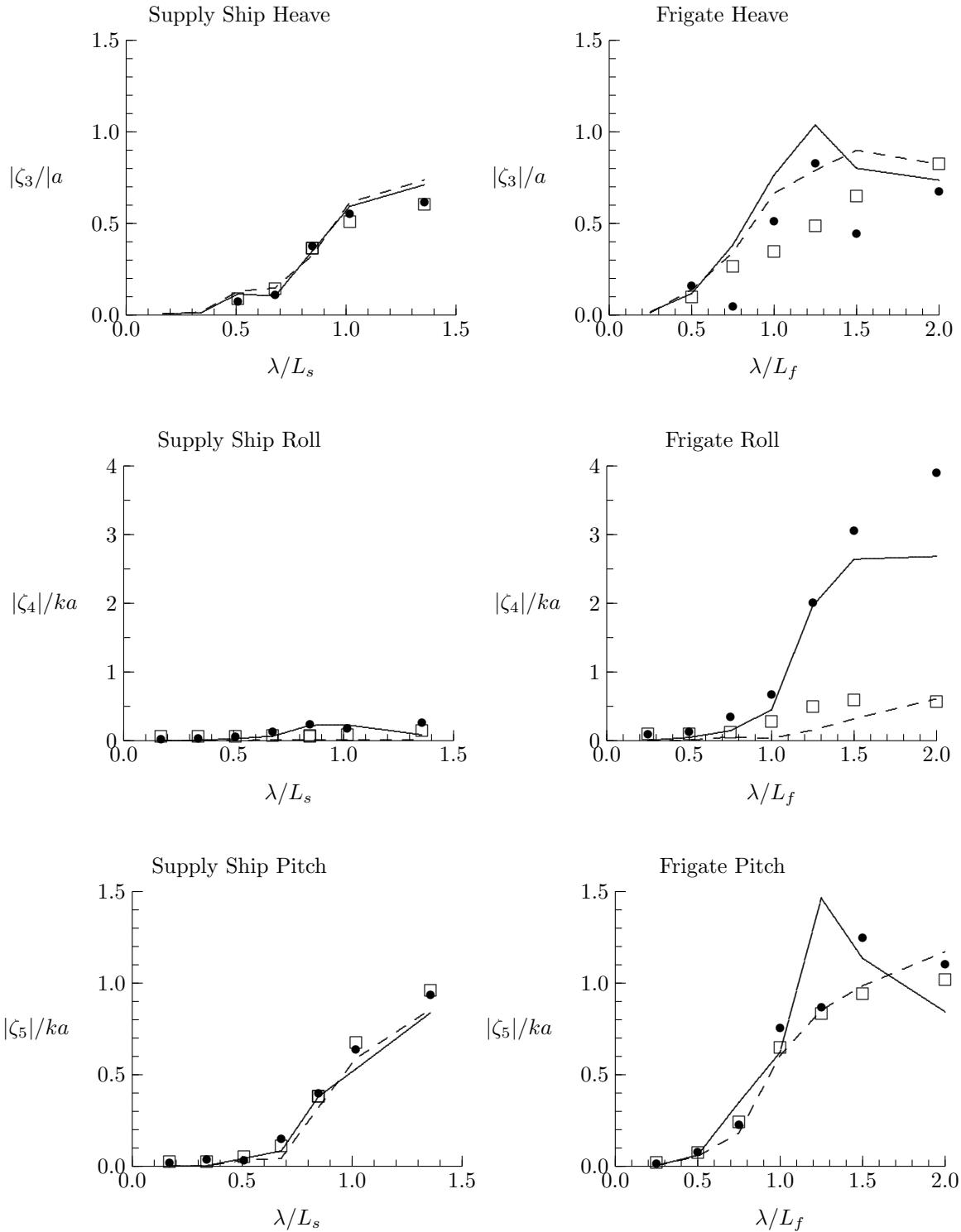
Figure 5: Ship Motions with Frigate Alongside Supply Ship, 12 knots, Head Seas
