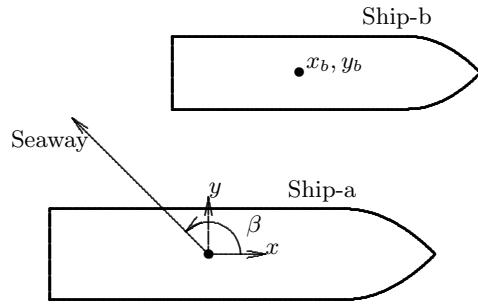
Figure 1: Plan View of Global Axis System
