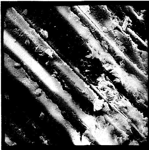
Figure 15 GRP sheet aged for 40 cycles in the Climate Lab ( \times 680 ).
