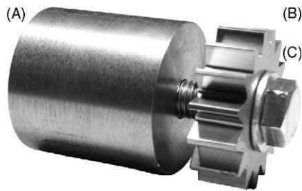
Fig. 1. Sample holder developed for green machining: (A) steel bar fixed in the chuck of the lathe to hold the sample, (B) sample to be machined and (C) tightening screw used to fix the sample on the steel bar.
