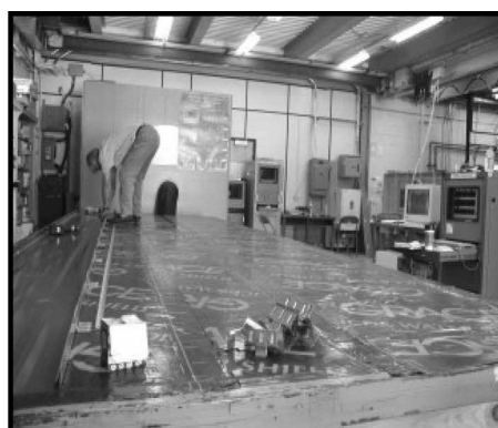
Fig. 7. Typical layouts of the air permeable deck condition with underlayment
