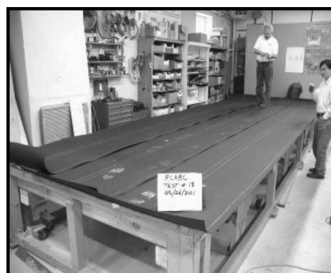
Fig. 7. Typical layouts of the air permeable deck condition with underlayment
