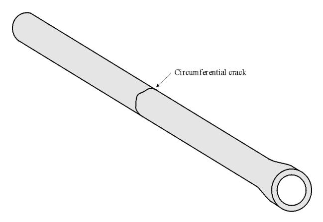
3. Circumferential failure. External bending forces in combination with corrosion pitting cause this form of failure.
