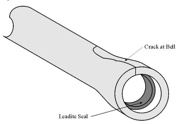
1. Split bell type failure, showing the bell end of the pipe. Differential thermal expansion between the bell and the leadite pipe seal causes this type of failure.
