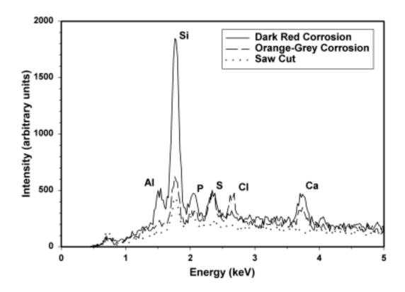
6. EDAX spectra of a pipe that had failed by a circumferential split. These spectra have been normalised against the iron  $K_{\alpha}$  signal.
