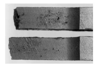
7. Pores in the machined surfaces of the Minneapolis pipe sample. These pores and the inclusions that accompanied them produced a pipe that was much weaker than is typical for its class of pipe.
