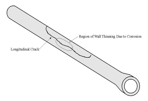
4. Longitudinal splitting. This type of failure is also caused by pipe wall thinning and pressure surges. The thinning can be produced corrosion or through pipe wall porosity. In some cases the crack will extend the length of the pipe.
