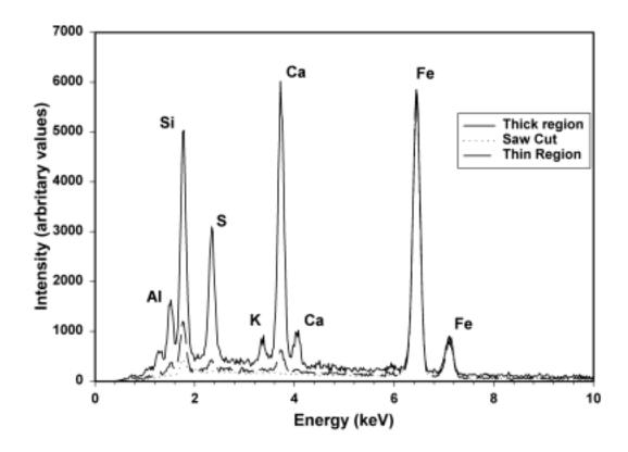
5. EDAX spectra of the pipe that had failed by a bell split. These spectra have been normalised against the iron  $K_{\alpha}$  signal.
