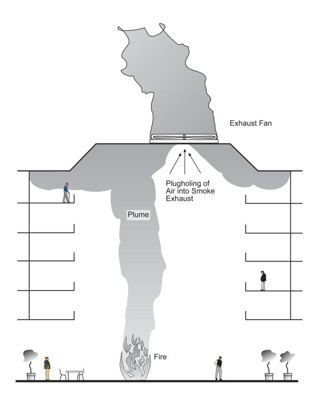
Figure 2. Pulling fresh air into the smoke exhaust resulting in plugholing.
