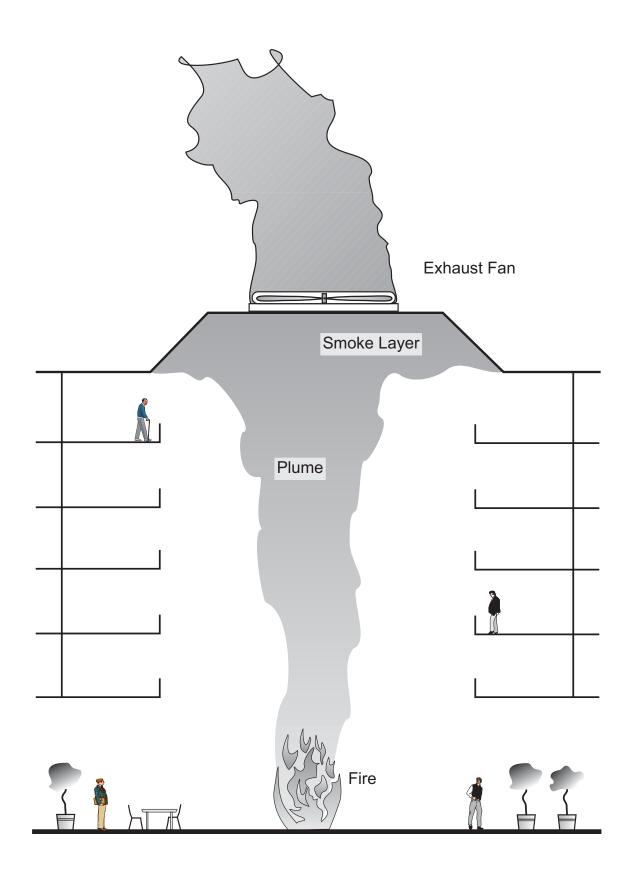
Figure 1. Smoke exhaust to maintain smoke layer above evacuation routes.
