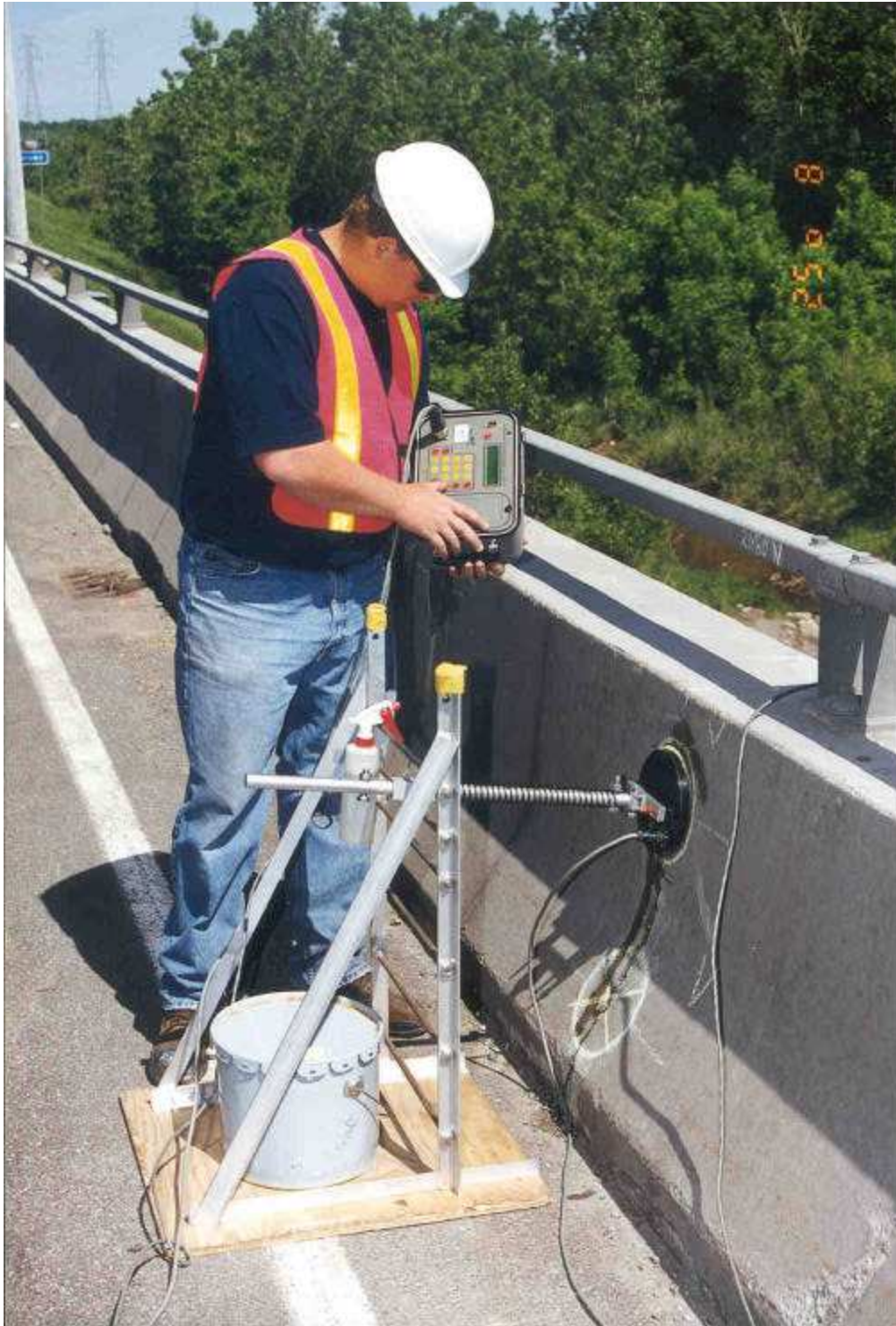
NRC technical officer measures the corrosion rate of the reinforcement in the barrier wall of the Vachon bridge.
