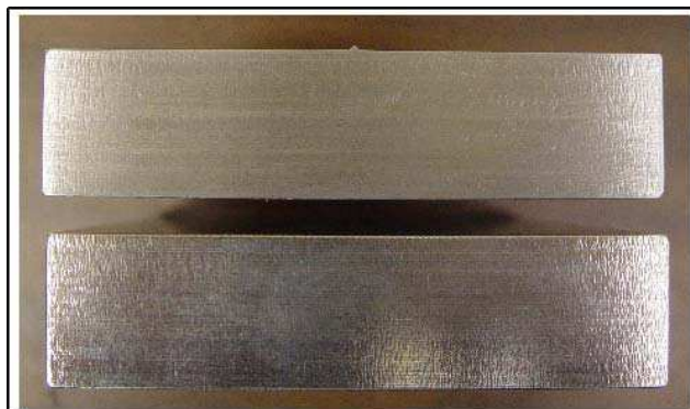
Figure 3. End views of the two aluminum plates used in the ice crushing experiments. The small triangular profile of the blade is visible on the top of the upper plate. The lower plate was bladeless.
