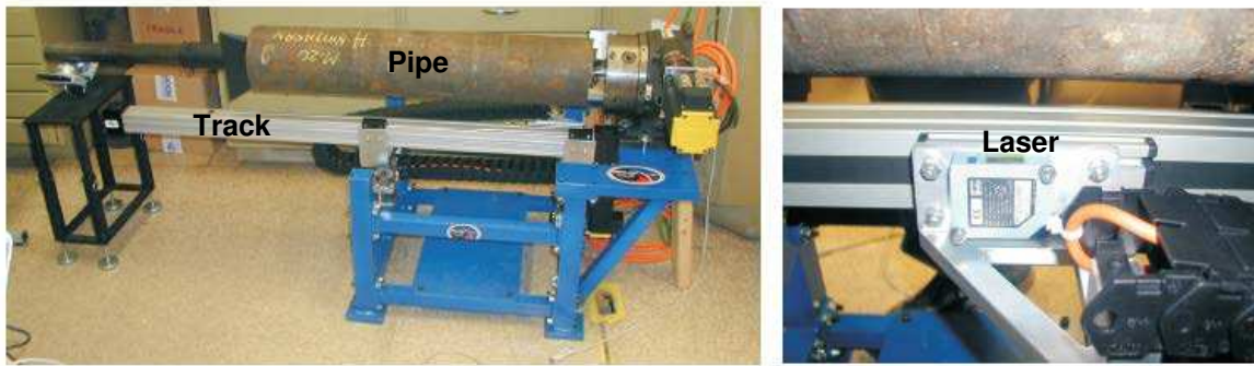
Figure 1. Pipe scanner (left: pipe mounted ready for scanning; right: laser point range finder mounted on track).
