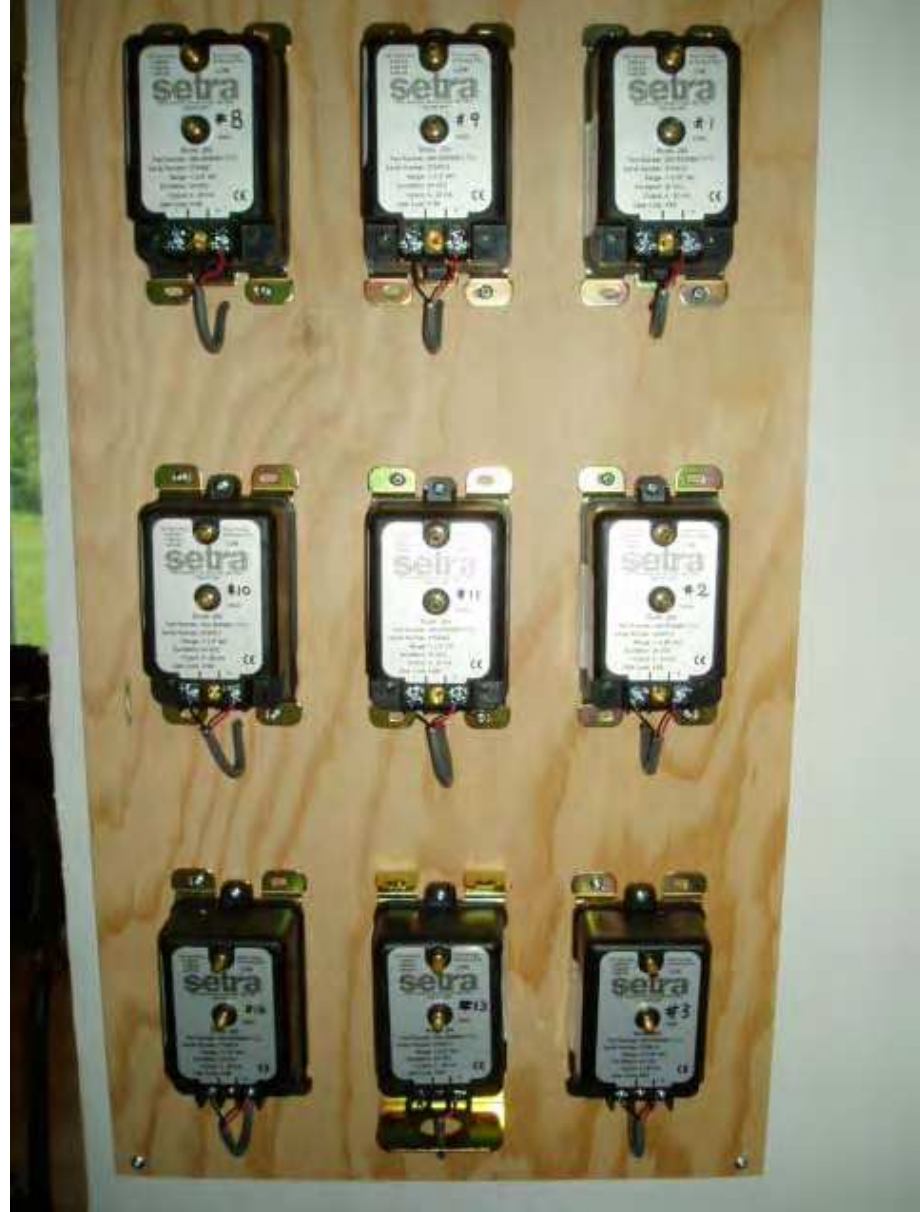
9 Differential Pressure Transducers: 3 DP of 0.25" WC 6 DP of 2.5" WC
