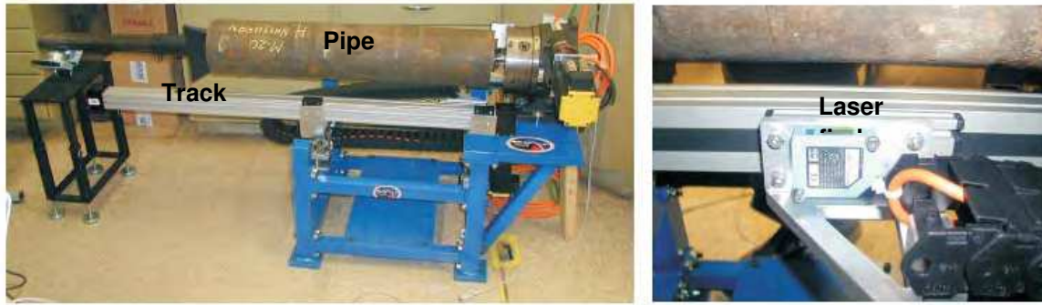
Figure 1. Pipe Scanner (left: pipe mounted ready for scanning; right: laser finder mounted on track).
