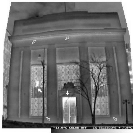
Figure 3 Thermographic scan superimposed on a video image. Arrows show points where air exfiltration is occurring (building pressurized for this test)
