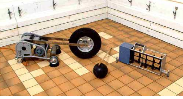
Figure 2: Standard impact sources, (from right to left) the ISO tapping machine, the Ball with a one-meter stick on it (dropping height) and the Bang Machine.
