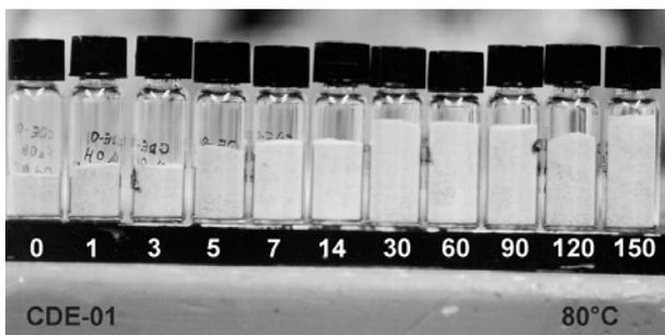
Figure 17. Picture of the ground Chinese limestone samples after various time periods of reaction at 80°C in 1M NaOH. Samples were filtered and washed with distilled water
