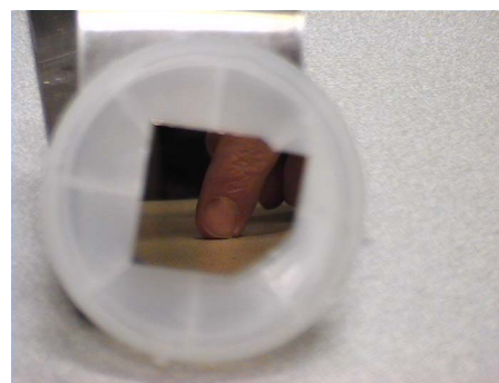
FIG. 2. Picture of a LaS thin film grown by PLD on a (100) Si substrate. The reflection of the finger clearly shows the metallic character of the thin film.
