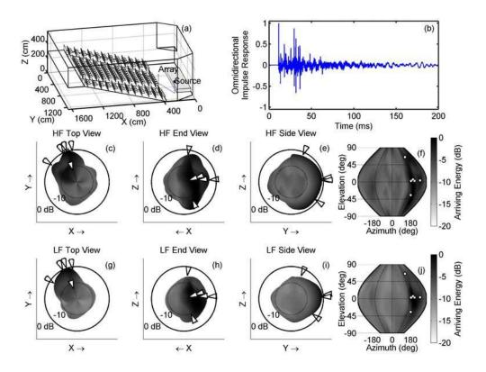
FIG. 10. Full decay time measurement in a small lecture theater. Layout is the same as Fig. 6.
