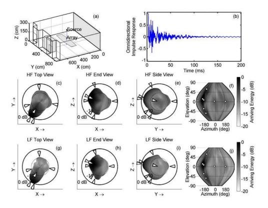
FIG. 9. Full decay time measurement in a videoconferencing room. Layout is the same as Fig. 6.
