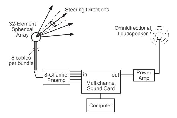
FIG. 1. Block diagram of measurement system. The microphone array steers a 28°-wide directional beam in 60 steering directions, detecting the sound arriving from each.
