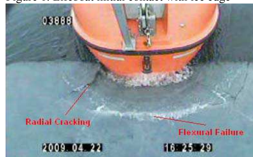
Figure 2. Ice failure due to flexure and compression
