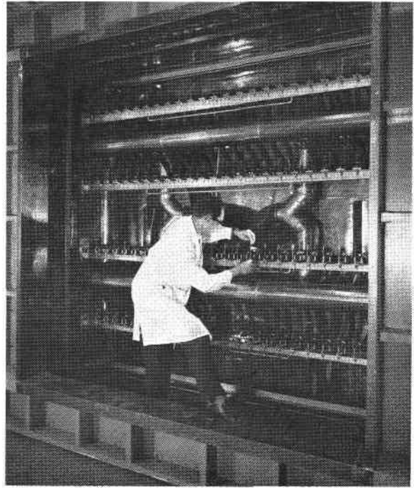
Fig. 4. Rain leakage apparatus, Division of Building Research of the National Research Council.
