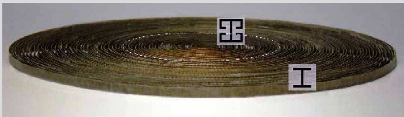
Image: An omnidirectional electromagnetic absorber made of metamaterials, © State Key Laboratory of Millimeter Waves, Department of Radio Engineering, Southeast University, Nanjing, China
