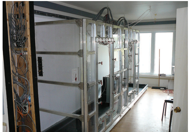
Figure 2. Interior of finished ICF walls and the climate control enclosure
