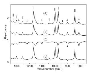
Figure 4. Illustration of the subtraction procedure for the PP film: (a) the MD spectrum; (b) the SF spectrum; (c) the difference spectrum MD –  $(1.29 \times SF)$ , multiplied by 3 to enhance the visibility; (d) the difference spectrum MD –  $(0.855 \times SF)$ , multiplied by 3.
