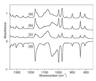
**Figure 5.** Illustration of the subtraction procedure for the film containing 2% clay and 4% E43: (a) the ND spectrum; (b) the SF spectrum; (c) the difference spectrum ND –  $(0.45 \times SF)$ ; (d) the difference spectrum ND –  $(2.56 \times SF)$ .
