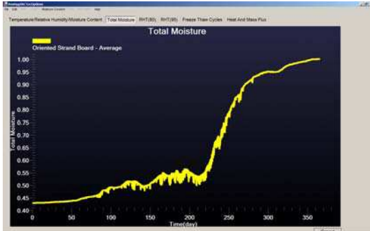
Figure 10. Output from 1-D hygIRC showing the variation of the total moisture content of one layer of the virtual wall through time (a time history).
