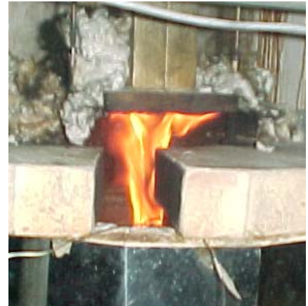
Figure 7: Burning of resin at 500°C, diameter 12.7mm GFRP sample
