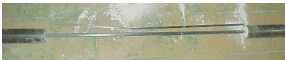
Figure 6: Failure mode of a 9.5 mm CFRP bar at ambient temperature
