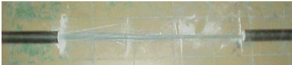
Figure 4: Failure mode of a 9.5 mm GFRP bar at ambient temperature
