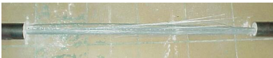
Figure 5: Failure mode of a 12.7 mm GFRP bar at ambient temperature
