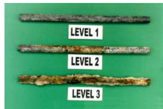
Figure 1. Rebar samples representing the 3 levels of corrosion observed.
