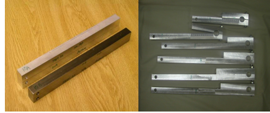
Figure 2: The finished aluminum and steel DCB (left) and aluminum CLS specimens (right) tested.
