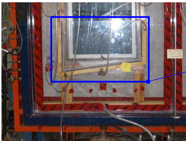
Figure 4 – Examples of water collection troughs; (a) collection trough for water draining from sill; (b) alternative trough configuration - water draining from sill; (c) collection trough for water that penetrates window (photo) and collection troughs for water penetration past the window, for drainage from the sill space, and for water drainage to the base of the wall (sectional sketch).
