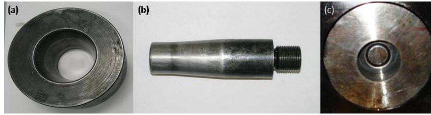
Figure 4. Tools utilized for variable thickness tube drawing: (a) die, (b) conical mandrel, (c) installed die and mandrel in the drawing machine.
