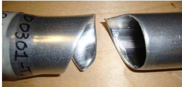
Figure 6. Fracture of the tube head with variable wall thickness
