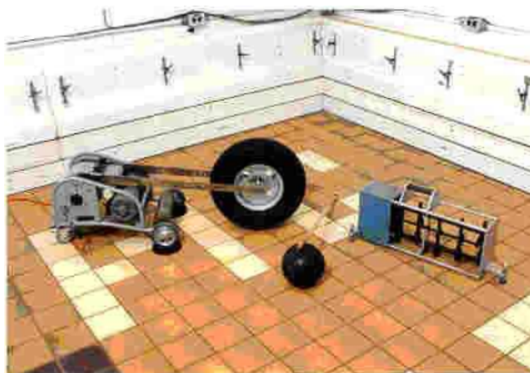
Figure 10. Photograph of 3 impact sound sources. From left to right are the Japanese tire drop machine, a resilient rubber ball and the standard tapping machine.
