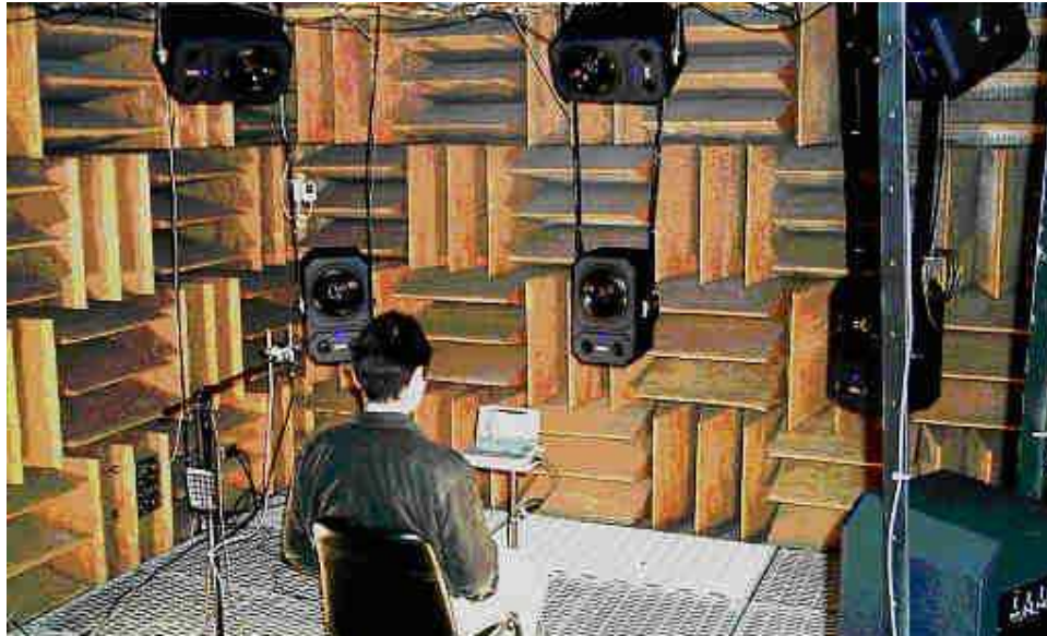
Figure 14. The room acoustics sound field simulation system in the NRC anechoic room.
