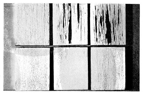
Figure 3—Cracking and peeling produced by cycle of three days of water immersion, three days of drying in twin carbon arc Weatherometer. Specification paint: top — commercial, bottom — laboratory.
