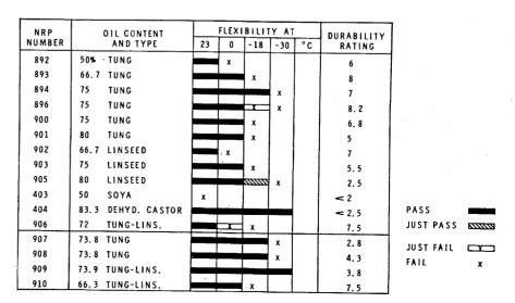
Figure 1-Low temperature flexibility.
