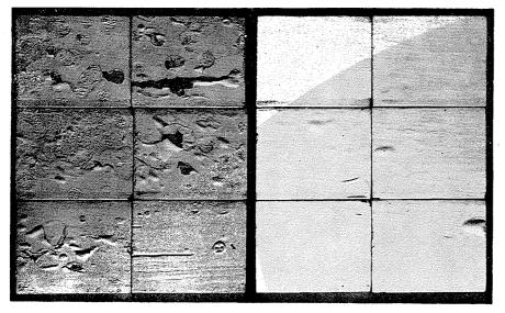
Figure 4—Blistering and cracking produced by cycle of 12 hours of light without water, 12 hours of water without light in single carbon arc Weatherometer. Specification paint: left — commercial, right — laboratory.
