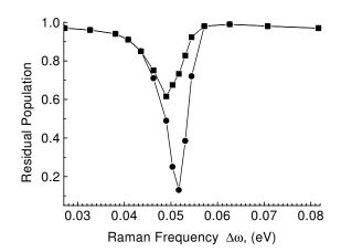
FIG. 4. Population of the v = 0 state (circles) and the total population of bound  $Cl_2^{3^+}$  states (squares) after the pulse  $\mathcal{E}f(t)[\cos(\omega_1 t) + \cos(\omega_2 t)]$  vs  $\Delta \omega = \omega_1 - \omega_2$ . The pulse parameters are  $f(t) = \sin(\pi t/T)$ , T = 1.2 psec (FWHM = 600 fs),  $\mathcal{E} = 5 \times 10^7$  V/cm,  $(\omega_1 + \omega_2)/2 = 1.17$  eV.
