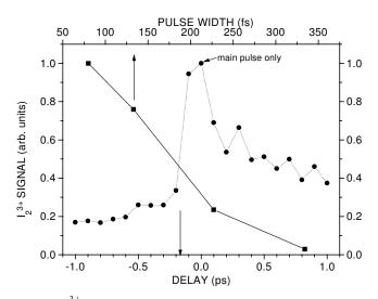
FIG. 3.  $I_2^{3^+}$  signal vs pulse duration (squares, solid line, top axis) or vs the time delay between the two 80 fs pulses (circles, dotted line, bottom axis). Negative (positive) delay corresponds to a pre-pulse (post-pulse). Intensity is  $3.6 \times 10^{14} \text{ W/cm}^2$  for the main pulse and  $1.2 \times 10^{14} \text{ W/cm}^2$  for the pre- or post-pulses.
