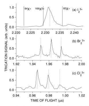
FIG. 1. Selected portions of the time-of-flight spectra showing peaks of  $I_2^{3+}$  (a),  $Br_2^{3+}$  (b), and  $Cl_2^{3+}$  (c). Dotted lines show anticipated positions of trications calibrated with well-known species. Positions of the singly charged mass 84 and 85 peaks and the position of the doubly charged mass 169 are included in (a) for reference.
