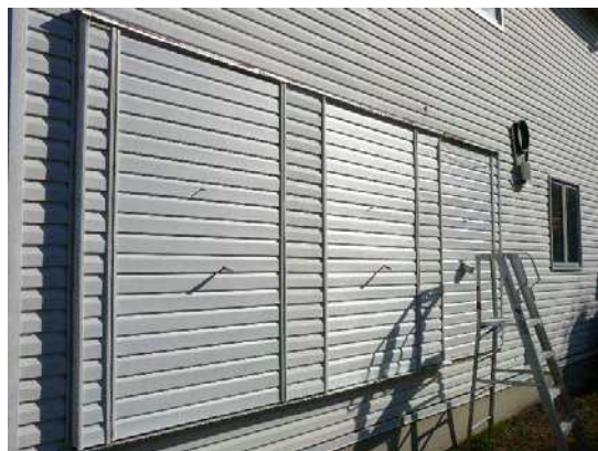
Figure 1: Field Exposure of walls facility and exterior view of the three test specimens
