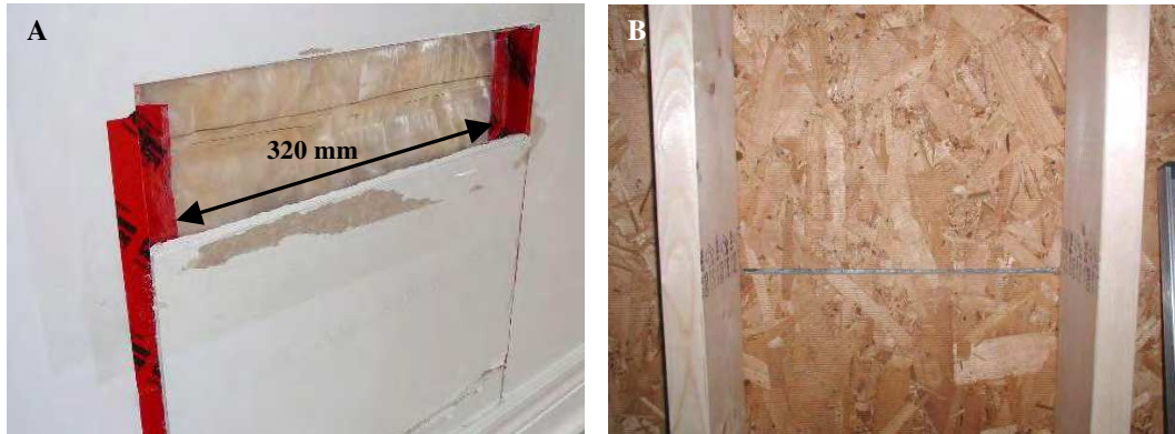
Figure 5: Air leakage openings A - Horizontal opening in the polyethylene membrane of 320 x 3mm. B- A 6 mm horizontal opening in the wood-based sheathing representing an open horizontal joint between panels
