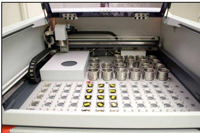
4 kW sequential WDXRF with end window and Rh-target X-ray tube
