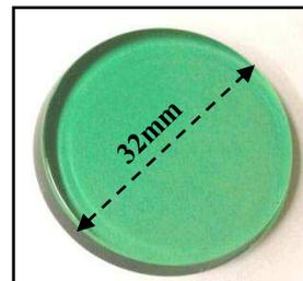
**Claisse 66.67%  $\text{Li}_2\text{B}_4\text{O}_7$ -32.83%  $\text{LiBO}_2$ -0.5%  $\text{LiBr}$**
