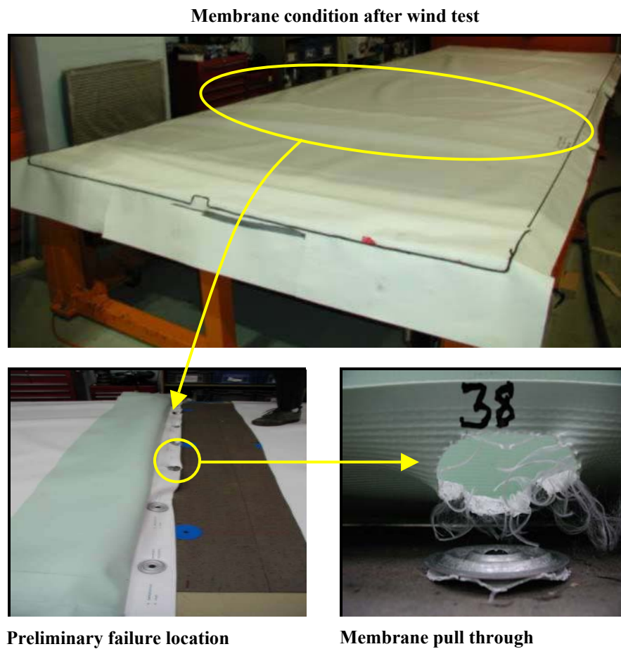
Figure 6: Failure mode of the tested system
