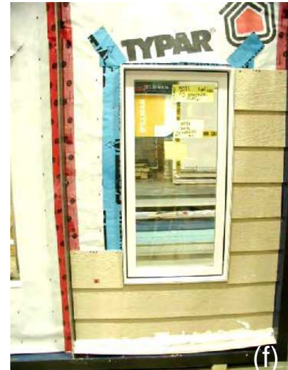
Figure 2 – (a) Schematic of specimen B-W1 showing B- and A-sides; (b) Sill pan PFP method B-side; (c) Proprietary drainage mat for B-side; (d) Lower portion of window on B-side prior to installation of drainage mat, cladding; metal clips support lower window flange; (e) Installation of WRB in rough opening of A-side prior to installation of window; shows lower portion next to sill; (f) A-side showing exterior cladding, and self-adhering flashing sheets at head (largely covered by flap in the WRB) and along one of the jambs.
