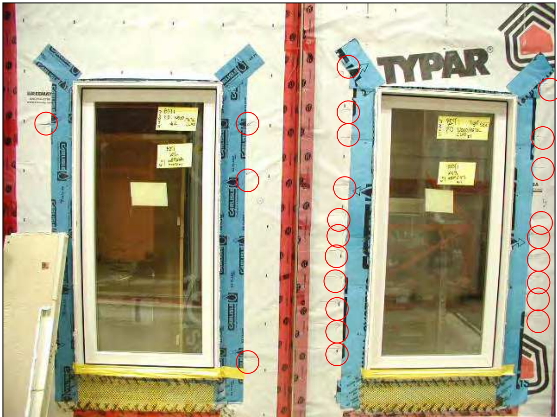
Figure 18 — Location of Fish Mouths on the B-side (left) and V-side (right) of B-W1
