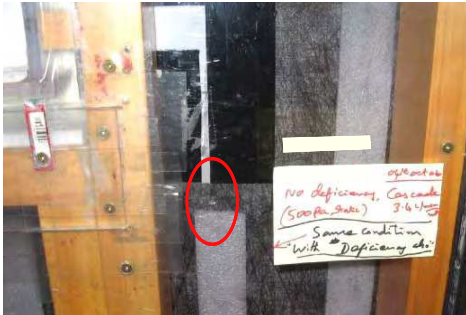
Figure 16 — B-W3 – Observed water leak behind WRB at the bottom corner of the window flashing; window installed before WRB; testing with no deficiencies
