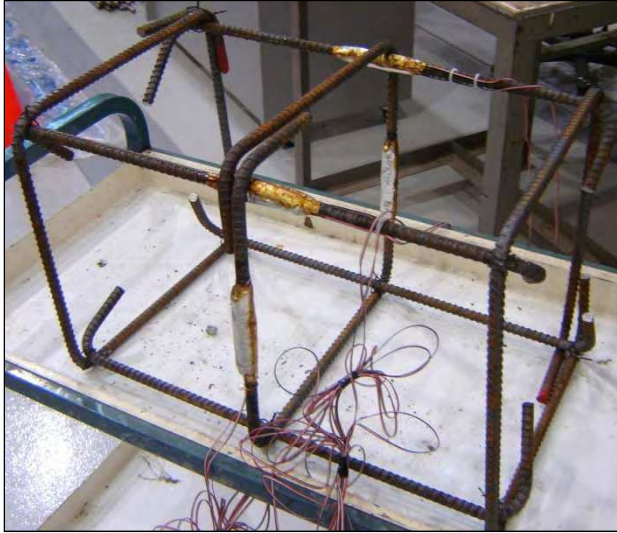
Figure 3. Electrical strain gauges applied on reinforcing bars (with protection).
