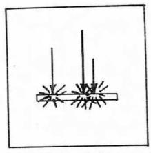
The conversion of radiant energy to heat energy is accomplished through a device commonly called a solar collector. A solar collector is either one of two types: a flat plate (or low temperature) collector, or a focusing (or high temperature) collector. Both type of collectors convert radiant energy, in most cases, to sensible heat. This sensible heat is characterized by a change in
