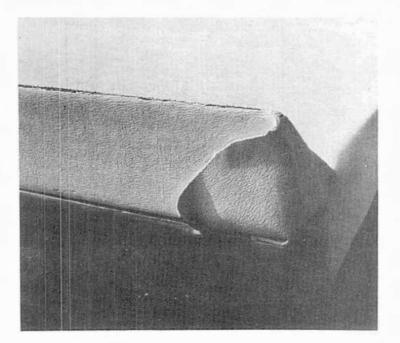
ROOF NO. 4 - 5 years exposure: severe chalking, splitting and checking.
