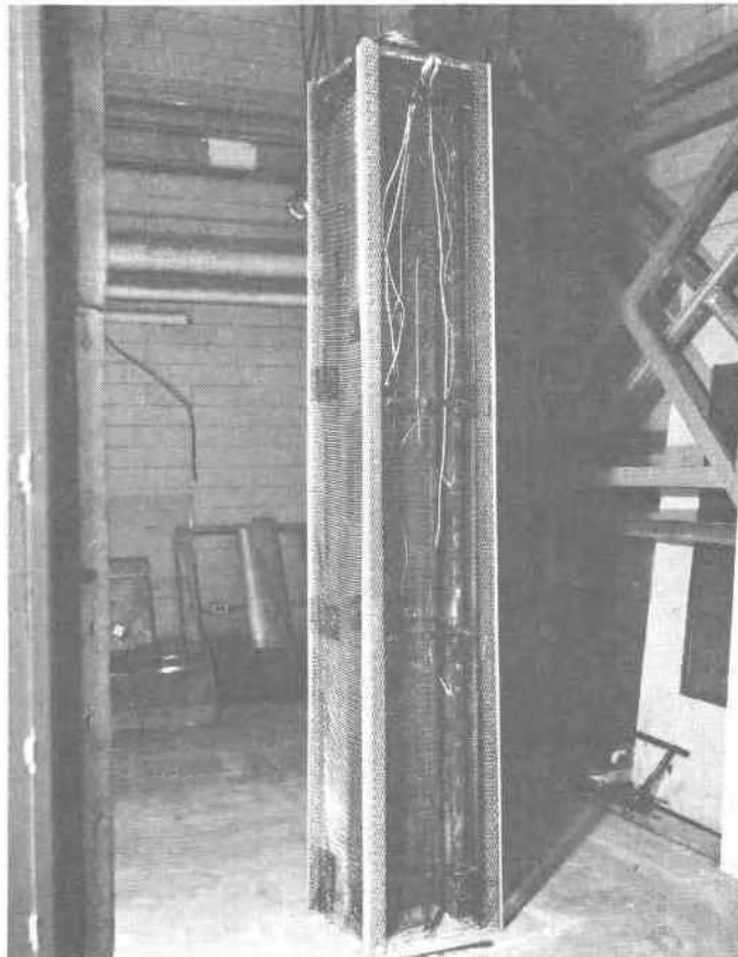
Figure 5 Column #7 Furred and Lathed.
